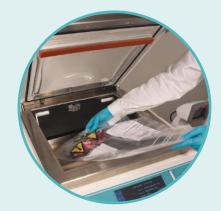
Place specimen in the vacuum bag and introduce it into the SealSAFE cavity. Close the lid.
