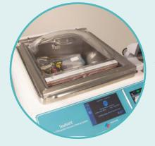
As a final step the SealSAFE vacuum seals the specimen bag. Fixative injection and sealing process are completed in the closed and ventilated cavity.
